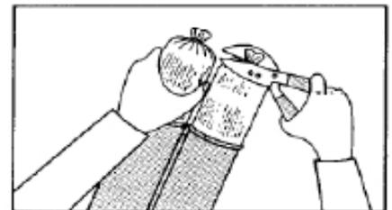
Cut off and remove the metal-clipped end of EZ-Pak sausage.
